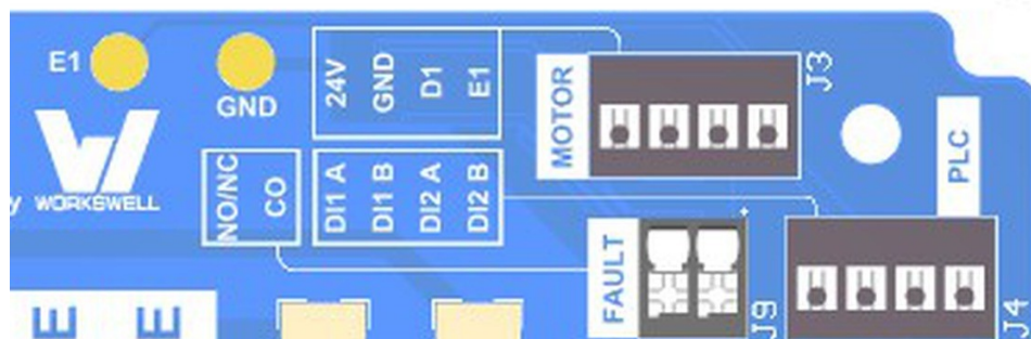
Figure 10: Location of the EC motor logic port (terminal blocks J3 "MOTOR" and J9 "FAULT") and of test points E1 and GND
